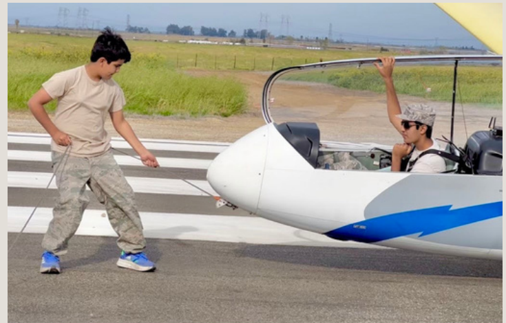
Cadet verifying that the tow line is securely connected to the glider hook. Photo by Lt Zafar Choudhry.
