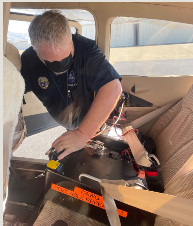
Major George Gadd checking installation of airborne repeater in aircraft.
