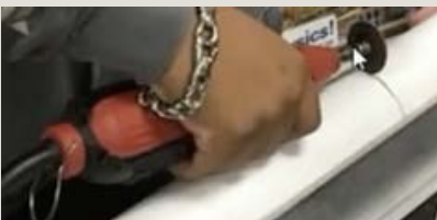
A cadet uses a Dremel tool to cut the fuselage of the rocket
