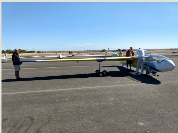
Volunteers assembling N420BA. First the right wing is joined to the fuselage. Photo by Lt Arnoldy
