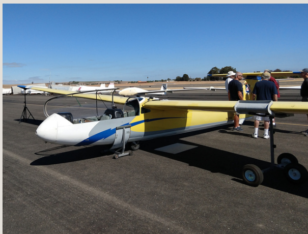
Volunteers assembling N420BA. The left wing is joined to the fuselage. Photo by Lt Arnoldy
