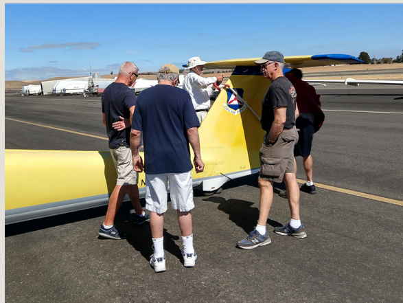
Volunteers assembling N420BA. The elevator is joined to the glider. Photo by Lt Arnoldy
