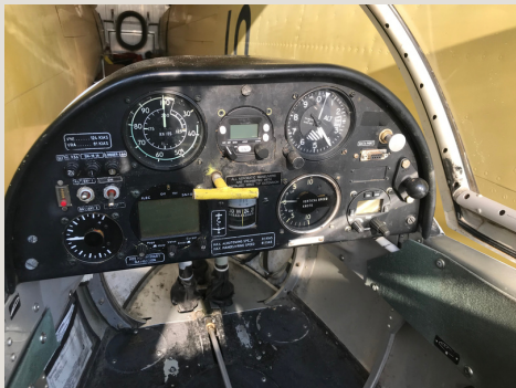
Glider front seat with the new ADS-B transponder in the front center.
