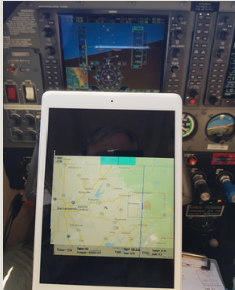
Pilot's iPad echoing Waldo System laptop display using "Duet" application. Photo by Capt S. Swale
