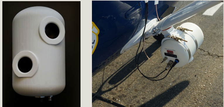
Figure 2. Left: the Ultra 50 pod from below, showing two cameras mounted at angles 45 degrees apart. Right: The Ultra 50 pod mounted on the right wing-strut, wired and ready to fly. (Photo: 1st LT A. Roudnev)
