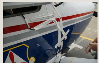
Figure 8. The wires from the Ultra 50 to the GPS unit and to the laptop inside the aircraft are taped to keep them from coming free. (Photo: 1st LT A. Roudnev)
